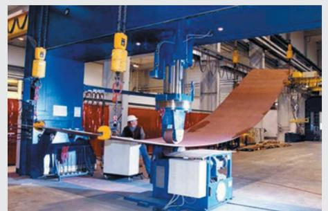
ship building press with mounted roll press unit
